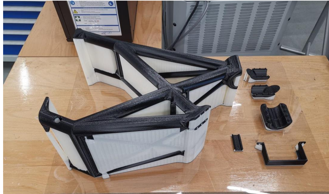
Figure 33. Printed frame and printed components
