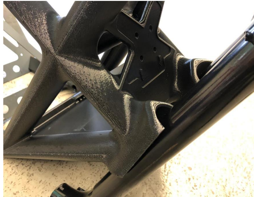
Figure 41. Gap between printed and metal frame
