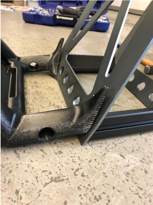
Figure 38. Down part where the metal tubes should be weld
